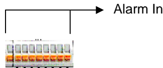
Figure 7 — Alarm Input connector strips.
