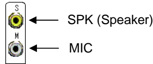
Figure 6 — Audio In and Out connectors.
